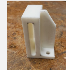
Replacement parts custom milled out of UHMW-PE
