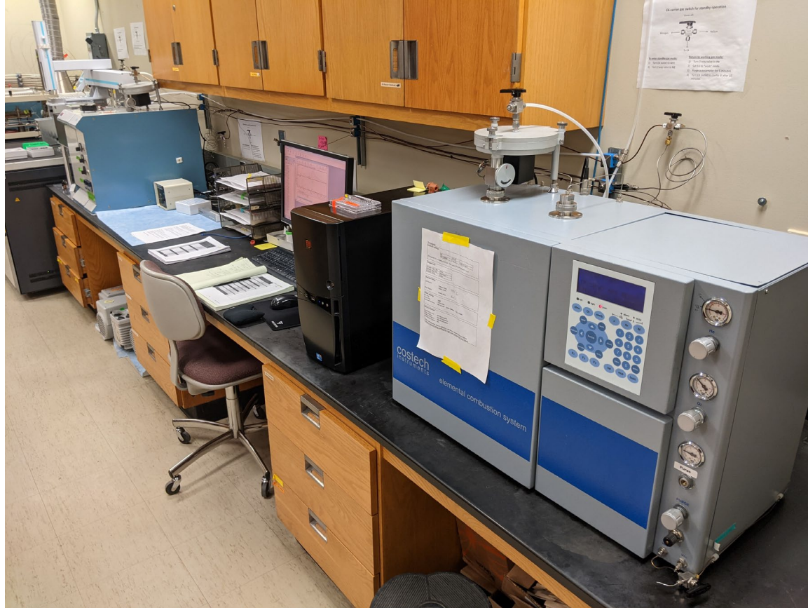
Costech 4010 elemental analyzer configured for CN or S quantification Thermo Pyrolysis elemental analyzer for H or O quantification
