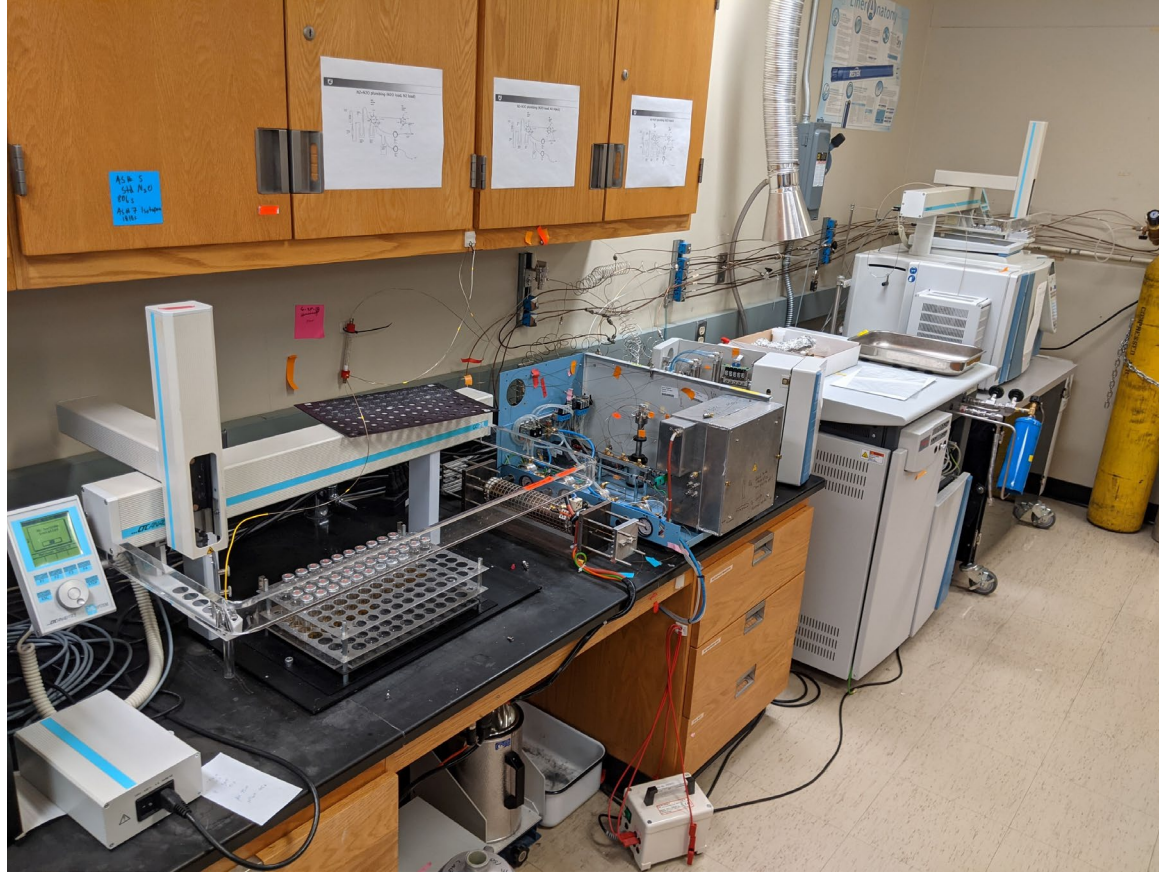
Modified Thermo Gas bench for nitrates, trace atmospheric gasses, N 2 O, N 2 O isotopomers, and GC for compound specific stable isotope analysis
